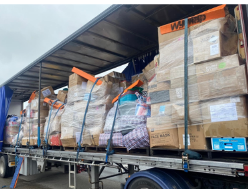
Wymap Group re-packed the loose cartons to pallets, shrink wrapped them, lashed for safe delivery and easy unpack at the Lismore Showground.
