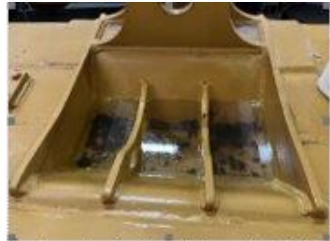
Pooling water in affected dozer blade (DAFF)
